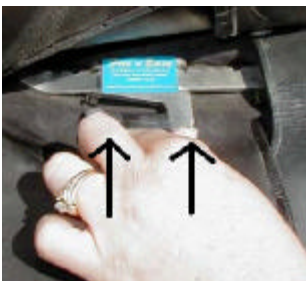
Push up against spring to release stirrup bar position
